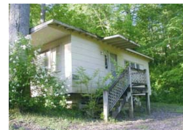
One of the A-6 prefabricated homes erected at Fontana Village in 1942 to house workers. These were the earliest forerunners of the modern mobile home
